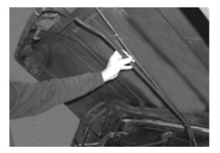
Route wires along hood support, and attached with the supplied clips. Be sure to protect wires along any sharp edges. Re-install hood support.
