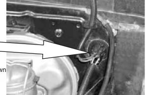
Trim wires to length and plug into the supplied connector, as shown below. Use the two single terminals for the It blue and dark blue wires. Use the double male terminal to crimp the two brown wires together.
