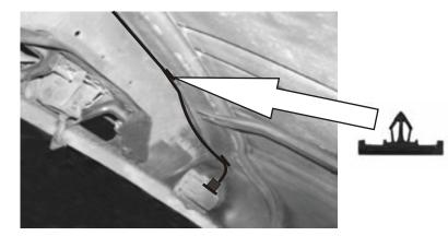
Attached the supplied clips to wires, and route all wires towards the driver side hood re-enforcement.
