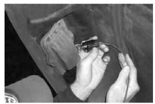
Plug the lamp socket with the It blue / brown into the driver's side lamp assembly, and the bk blue / brown into the passenger side.
